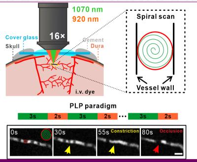
Figure 2 Illustration of the Precision 1070 nm Ultrafast Laser-induced Photothrombosis (PLP) of Depth-targeted Vessels
